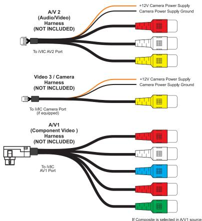
as Input Signal Type, then you must use Green connector for Composite Video
