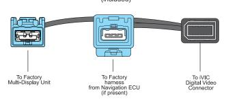
Digital Video Cable MUST BE CONNECTED to Factory Multi-Display Unit, Navigation ECU (if present), and to iVIC for proper operation of iVIC and factory components.
